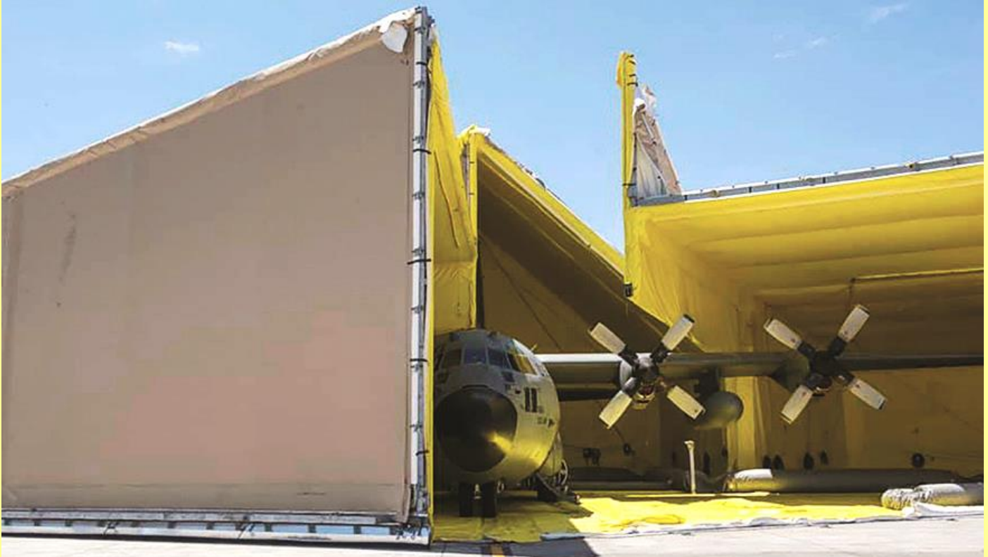
The Joint Biological Agent Decontamination System (JPO CBRN Defense photo)
