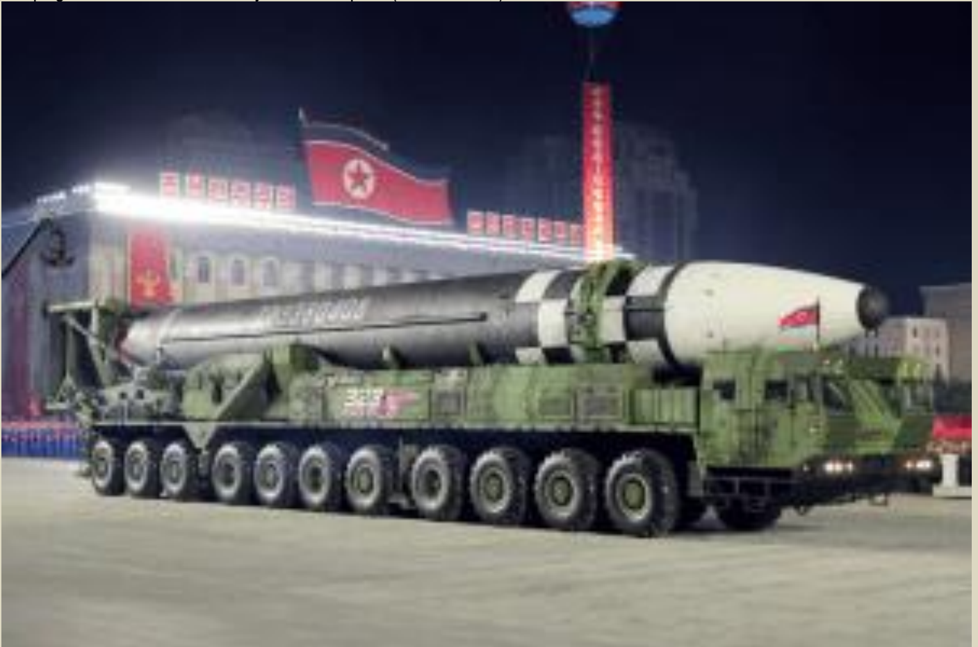
Figure 2: The Hwasong-16 ICBM was first displayed at the October 2020 parade in Pyongyang. The missiles, which is carried on an 11-axle transporter erector-launcher (TEL), has not been flight tested. (Image: North Korean government).
