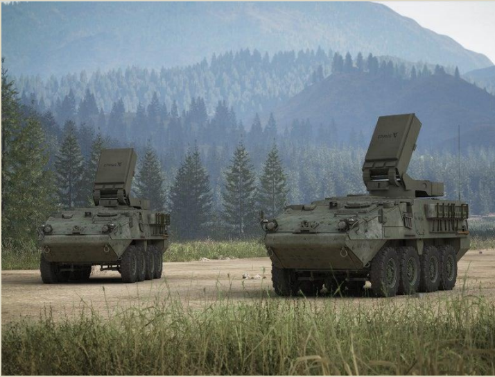
The Leonidas system can be mounted on top of the US Army's Stryker armored vehicle. Credit: Epirus, Inc.
