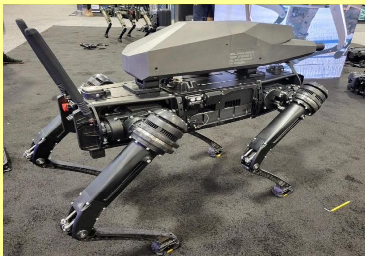
Special Purpose Unmanned Rifle, or SPUR on Spot’s back
