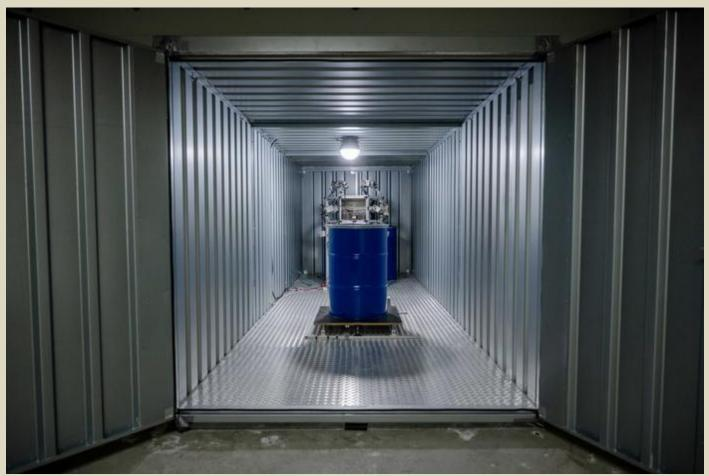
In this container, the researchers tested how robust and how reproducible the radio fingerprint is. The technology detects movements of the blue barrel.
