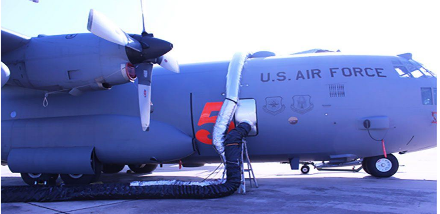
In this 2020 photo, the Joint Biological Agent Decontamination System (JBADS) is being used on a C-130 airplane interior to extinguish mold. Credit: Donna Lindner, Air Force Research Laboratory
