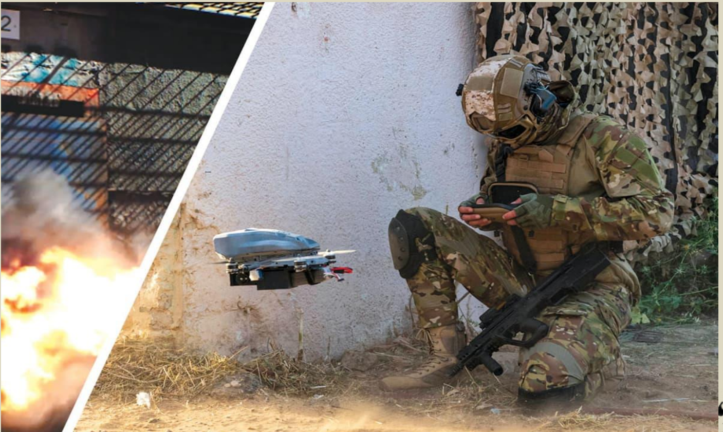
A lethal search, map and destroy combat drone capable of operating autonomously, either alone or in swarms (Elbit Systems)
