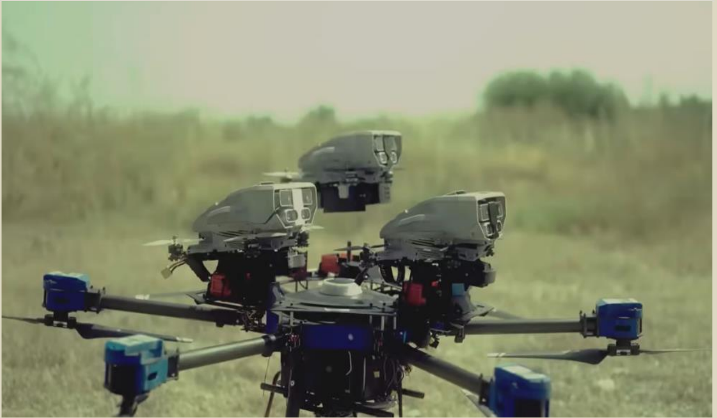
Up to three Lanius drones can ride on the back of a mothership drone, or they can be physically carried by operators in the field (Elbit Systems)
