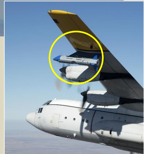
An X-61 Gremlin Air Vehicle (GAV) engages the "recovery bullet" of a C-130 Hercules aircraft (DARPA)
