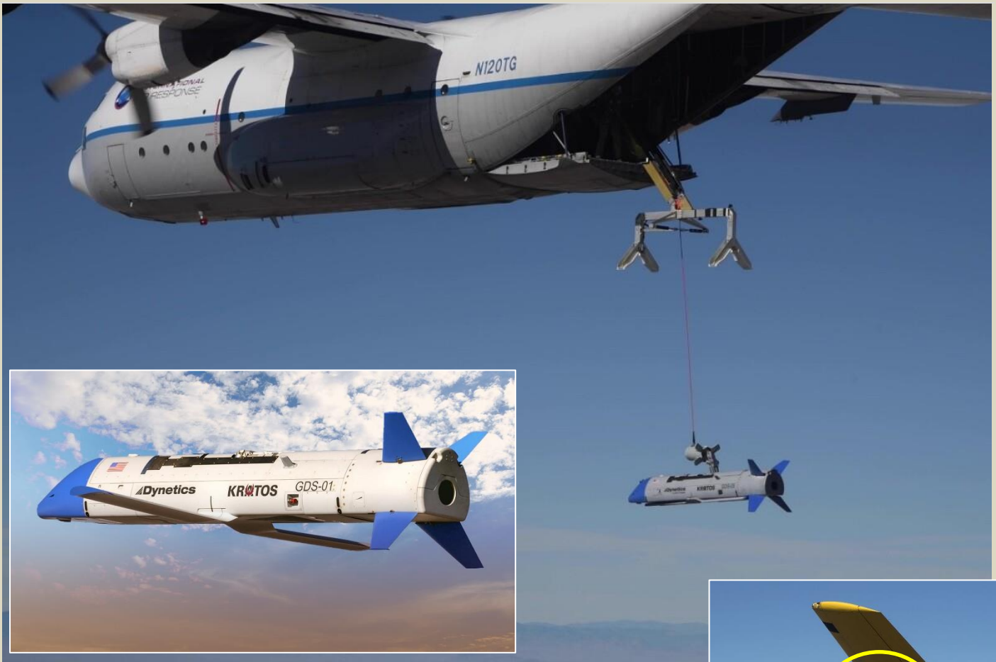
An X-61 Gremlin Air Vehicle (GAV) engages the "recovery bullet" of a C-130 Hercules aircraft (DARPA)
