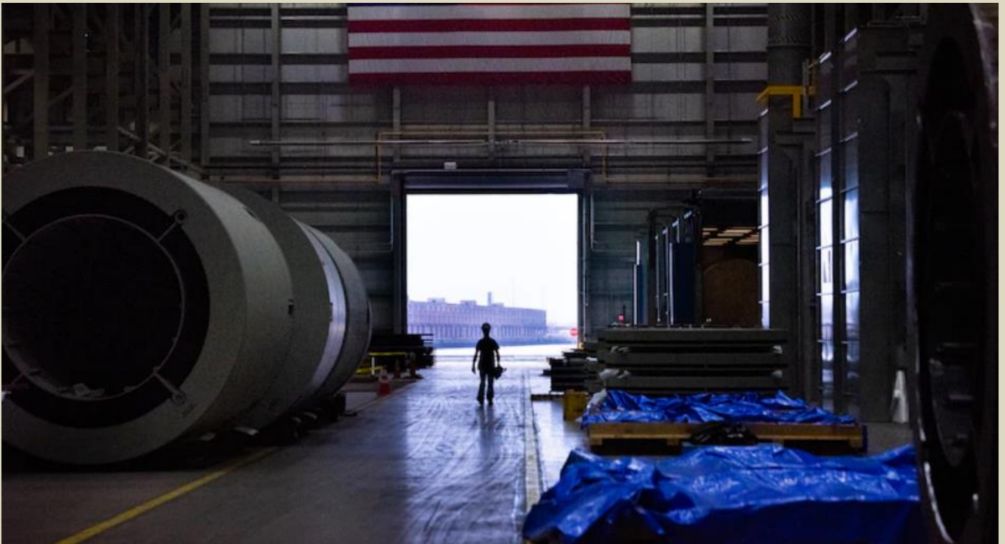
A worker at Holtec International's manufacturing plant in Camden, N.J. On the left are steel canisters used to store nuclear waste for decades. (Sarah L. Voisin)
