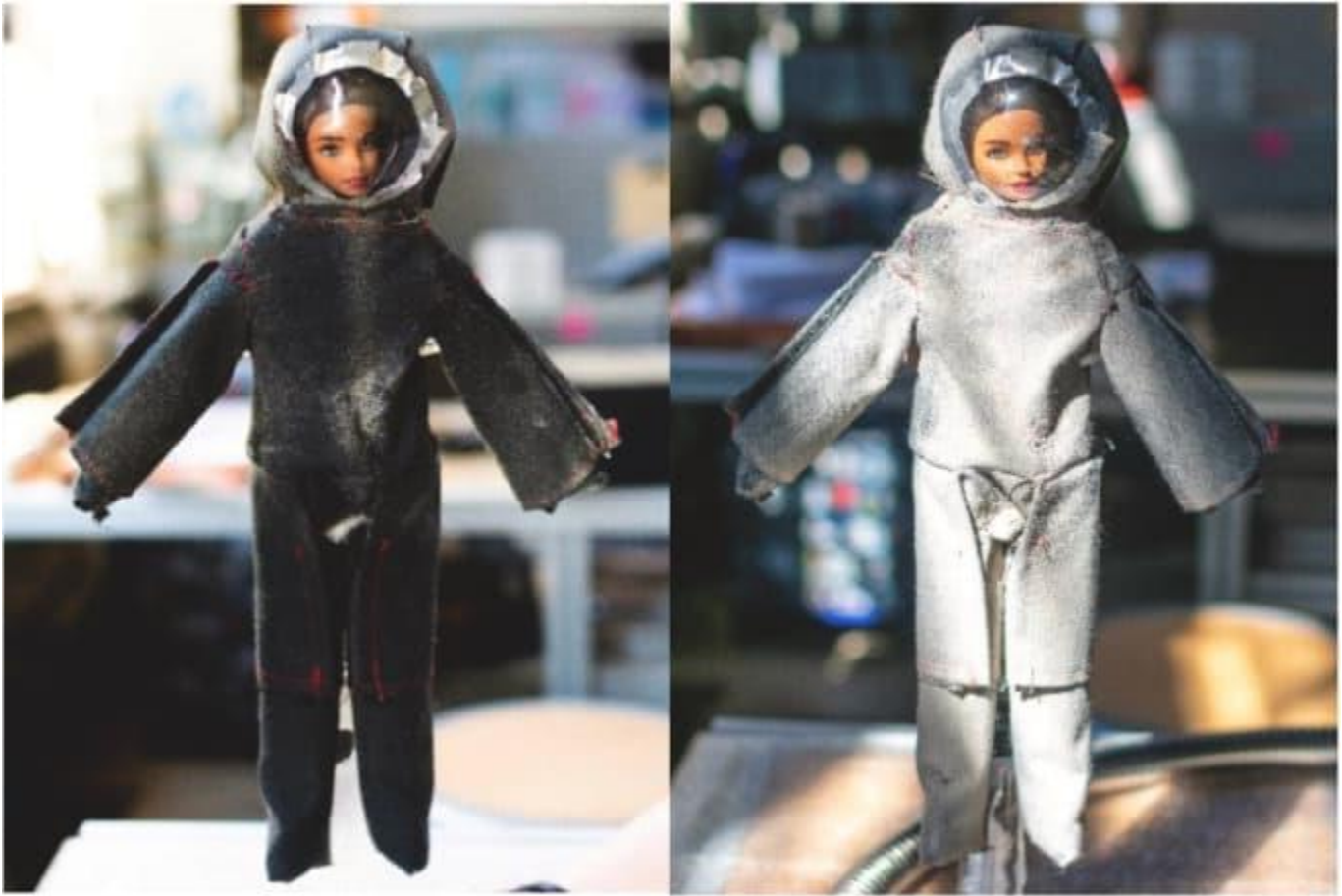
A sample of black material covered in gray dust before (left) and after the liquid nitrogen treatment in a vacuum – Washington State University
