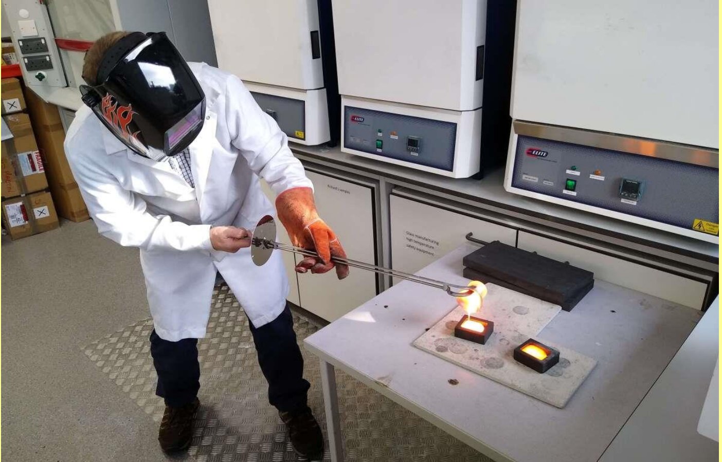
Samples of the glass are poured in the lab (Aston University)
