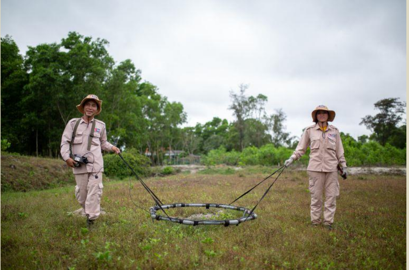
MAG staff use a loop detector to search for unexploded ordnance in Trieu Phong District [Chris Humphrey/Al Jazeera]
