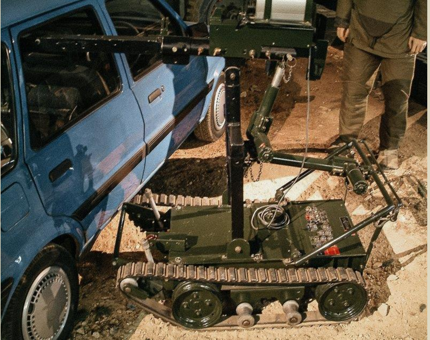
The Wheelbarrow remotely controlled bomb disposal tool developed during the Troubles conflict in Northern Ireland in the 1970s. Wikimedia Commons photo.
