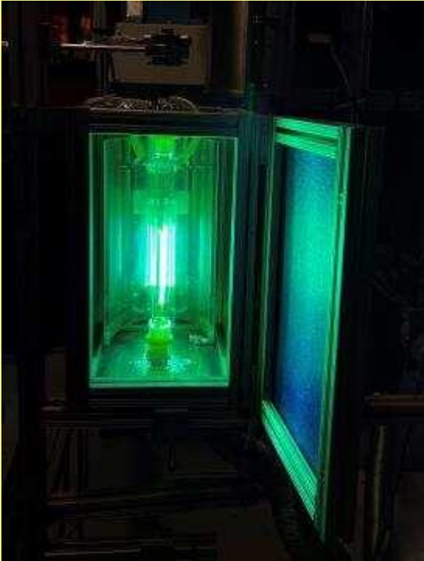
Ultraviolet lamp used for curing the wire cladding. Photo credit: University of Massachusetts Lowell.
