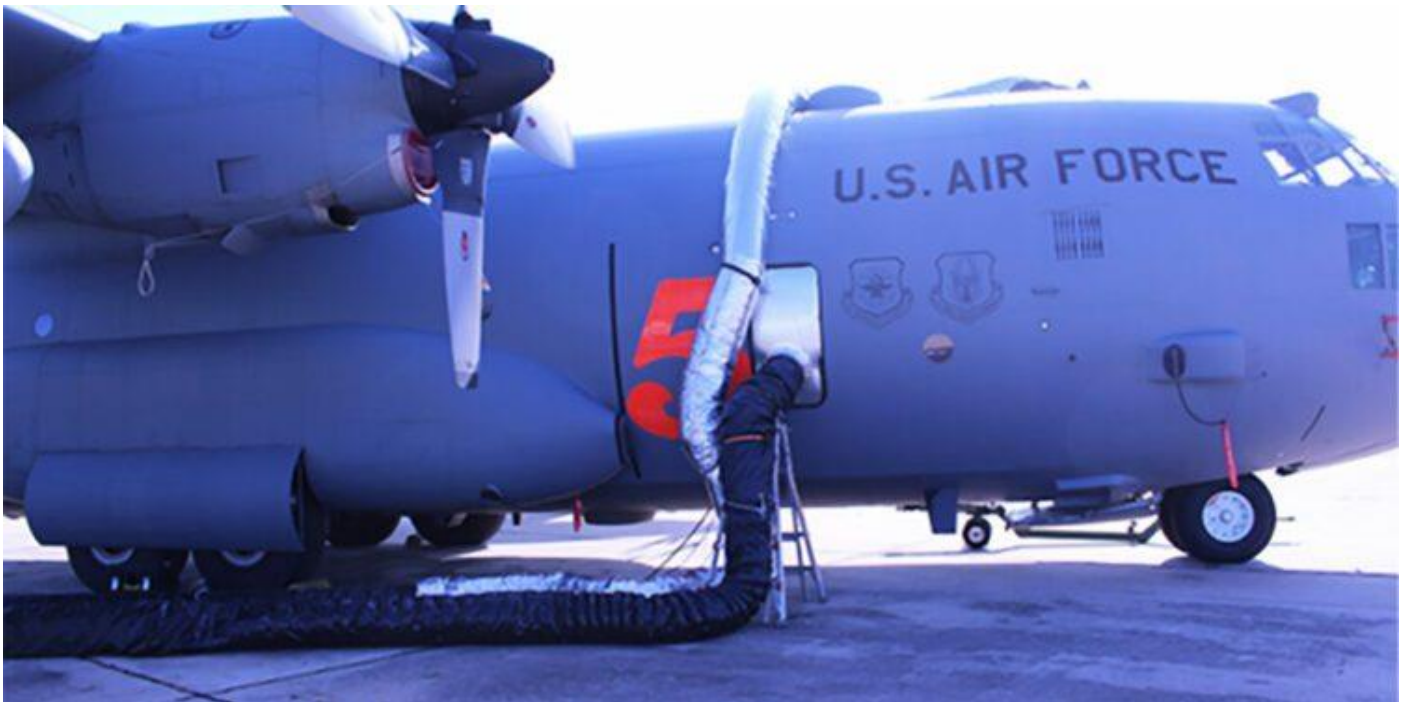
In this 2020 photo, the Joint Biological Agent Decontamination System (JBADS) is being used on a C-130 airplane interior to extinguish mold. Credit: Donna Lindner, Air Force Research Laboratory
