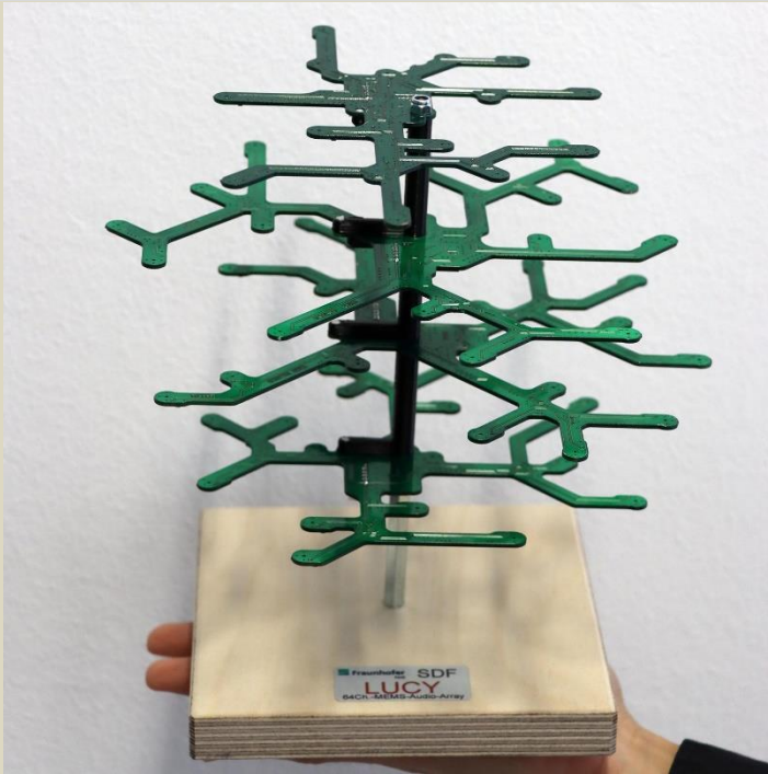
The present version of LUCY, which incorporates 48 MEMS microphones | Fraunhofer FKIE
