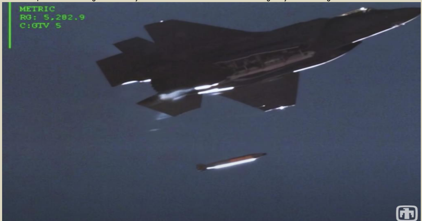
A US F-35A combat aircraft tests an unarmored B61-12 bomb in the Nevada Desert. Source: Sandia National Laboratory
