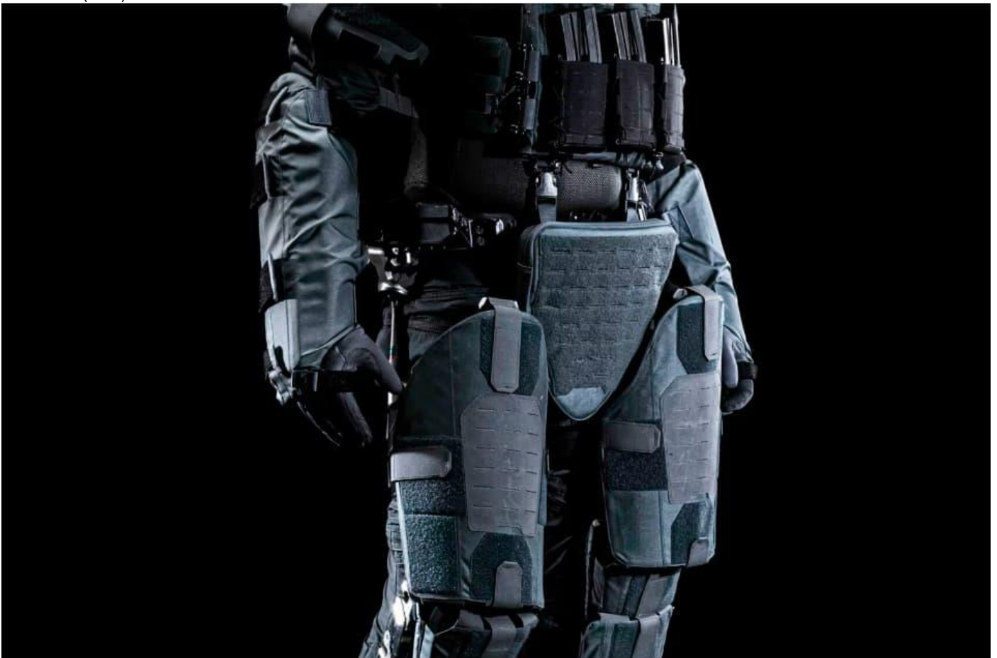
Body armor panels are located throughout the exoskeleton - Mehler Protection
