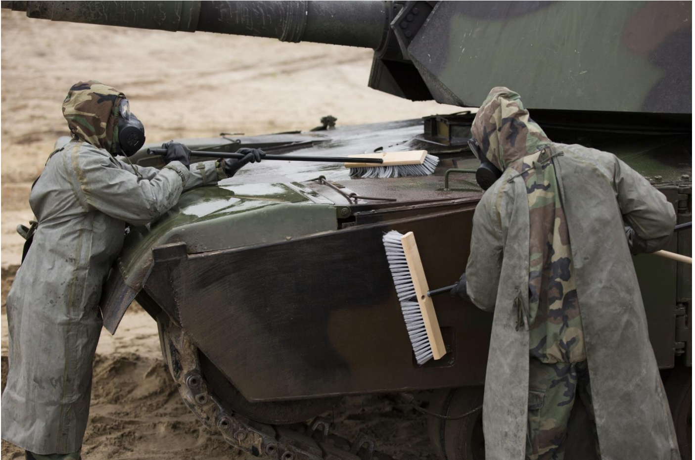
Decontamination is part of AFV CBRN survivability. (Photo: USMC)
