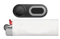
If things continue to escalate, the user presses the button a second time. This makes the ring turn red, and it causes the PhoneCam to start transmitting footage to a cloud-based server, where it's recorded for possible use in court or by the police.
