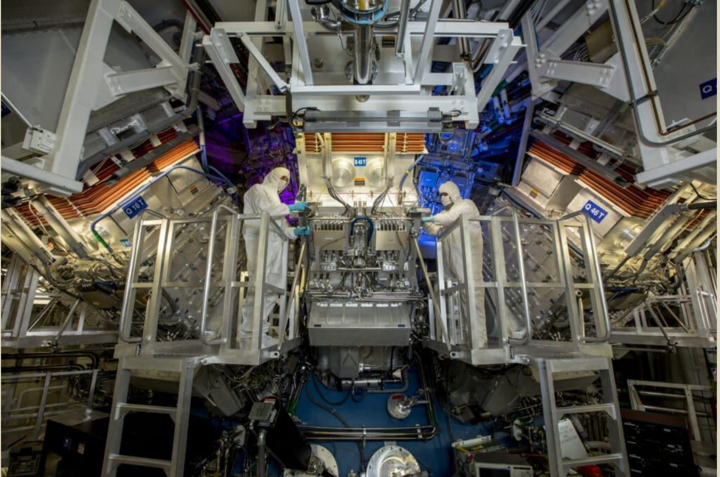
National Ignition Facility operators inspect a final optics assembly during a routine maintenance period in August. Photo credit: Lawrence Livermore National Laboratory
