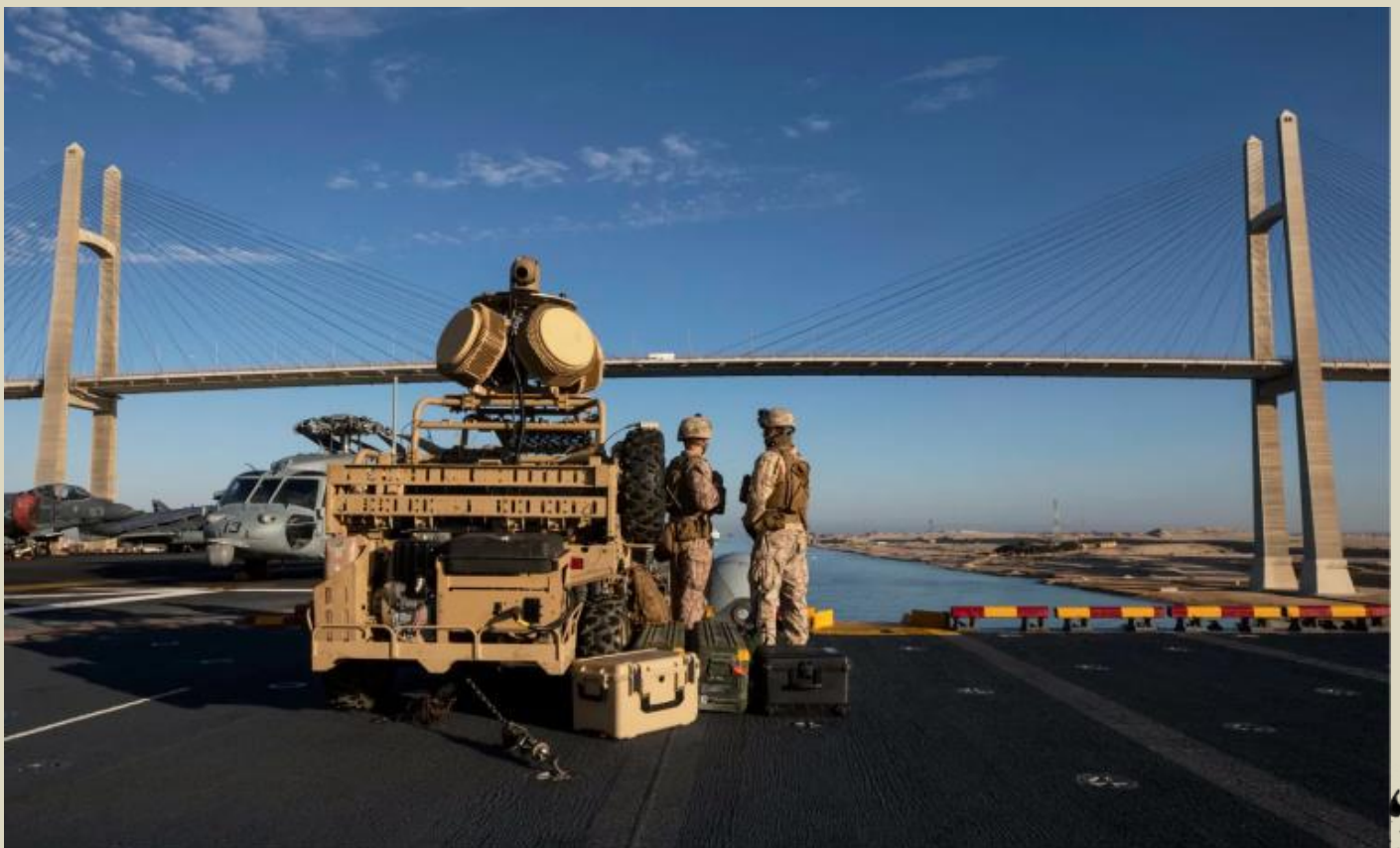
The LMADIS uses two Polaris MRZRs, one acting as the brain and the other as the brawn. Together, they house the CM262U optic, which acts as the ‘eyes’ of the system; the RPS-42 radar and Skyview MP,
