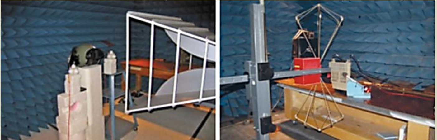
Figure 2: (left) EOD helmet tested for electromagnetic compliance (MIL-STD-461 and Def-Stan59-411) in an anechoic chamber (David Florida Laboratory, Canadian Space Agency, Ottawa, Ontario, Canada) (right) RF jammer (Allen-Vanguard) subjected to the same tests.
