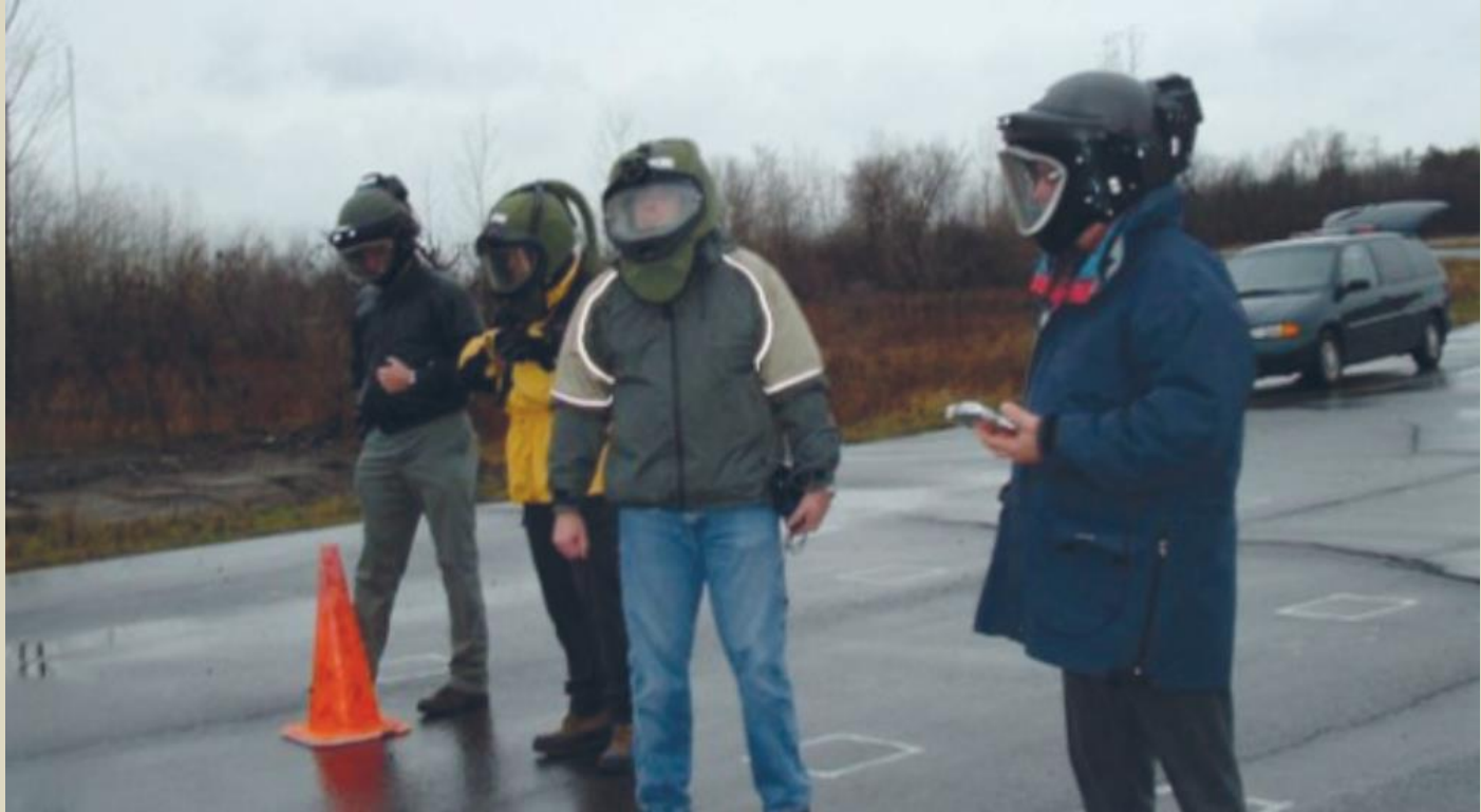
Figure 4: Volunteers testing the functionality of different Med-Eng legacy EOD helmets at varying distances from an ECM device.
