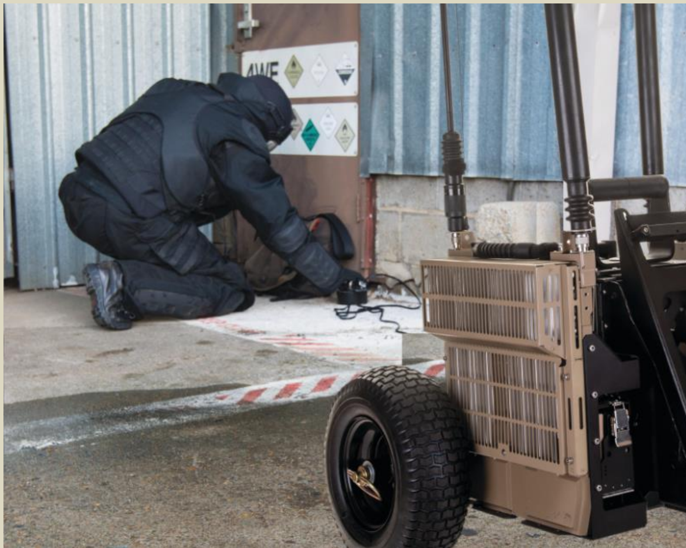
Figure 3: RF jammers in close proximity (SCORPION, Allen-Vanguard) on a “Dual Carrier” to maximize the jamming response for enhanced operator safety.
