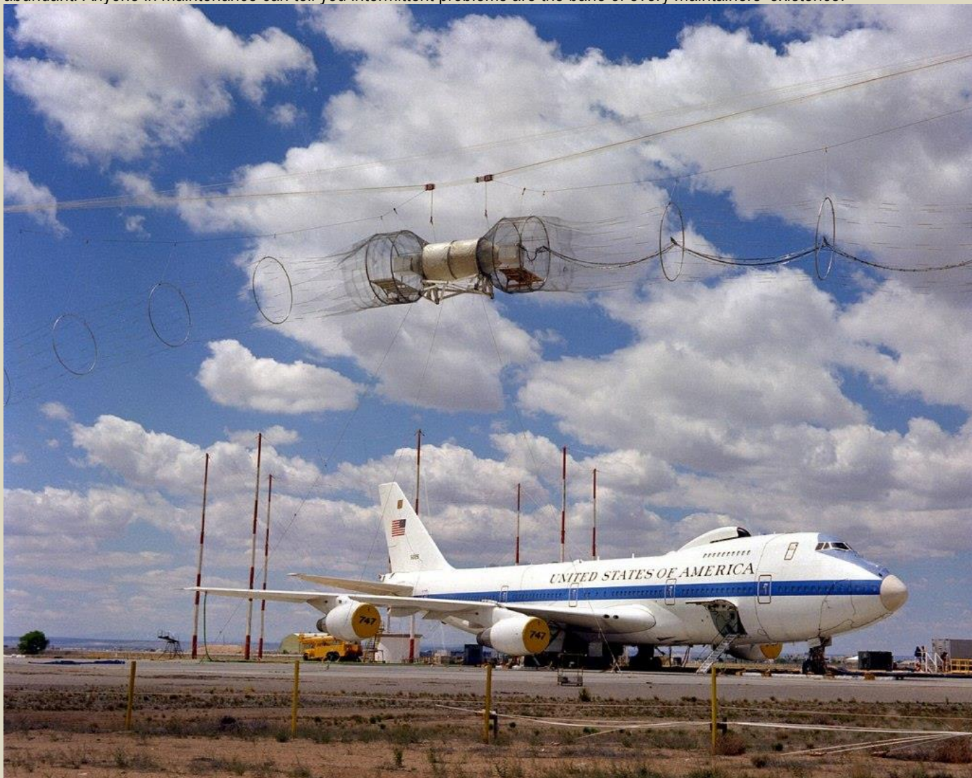
A right front view of an E-4 advanced airborne command post (AABNCP) on the electromagnetic pulse (EMP) simulator for testing. (Photo by Sgy Ernie Stone/U.S. Army)
