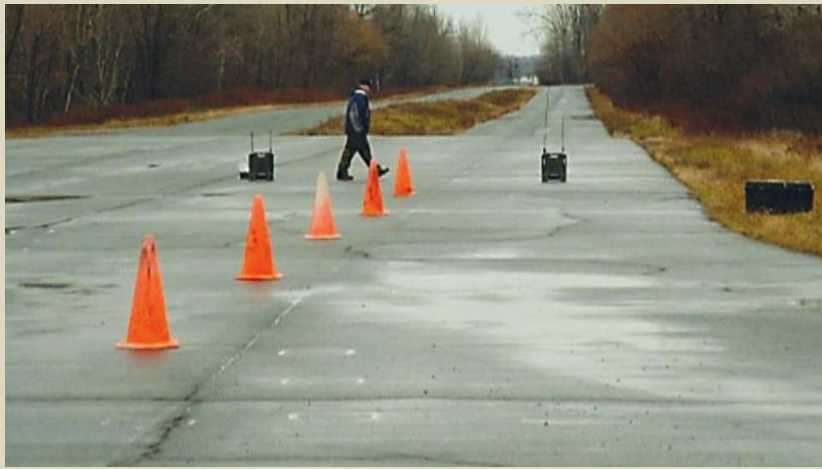
Figure 5: Test setup for the EOD helmet tests against actual jammers. Pylons positioned at 10-meter intervals from two SCORPION ECM devices (Allen-Vanguard jammers).
