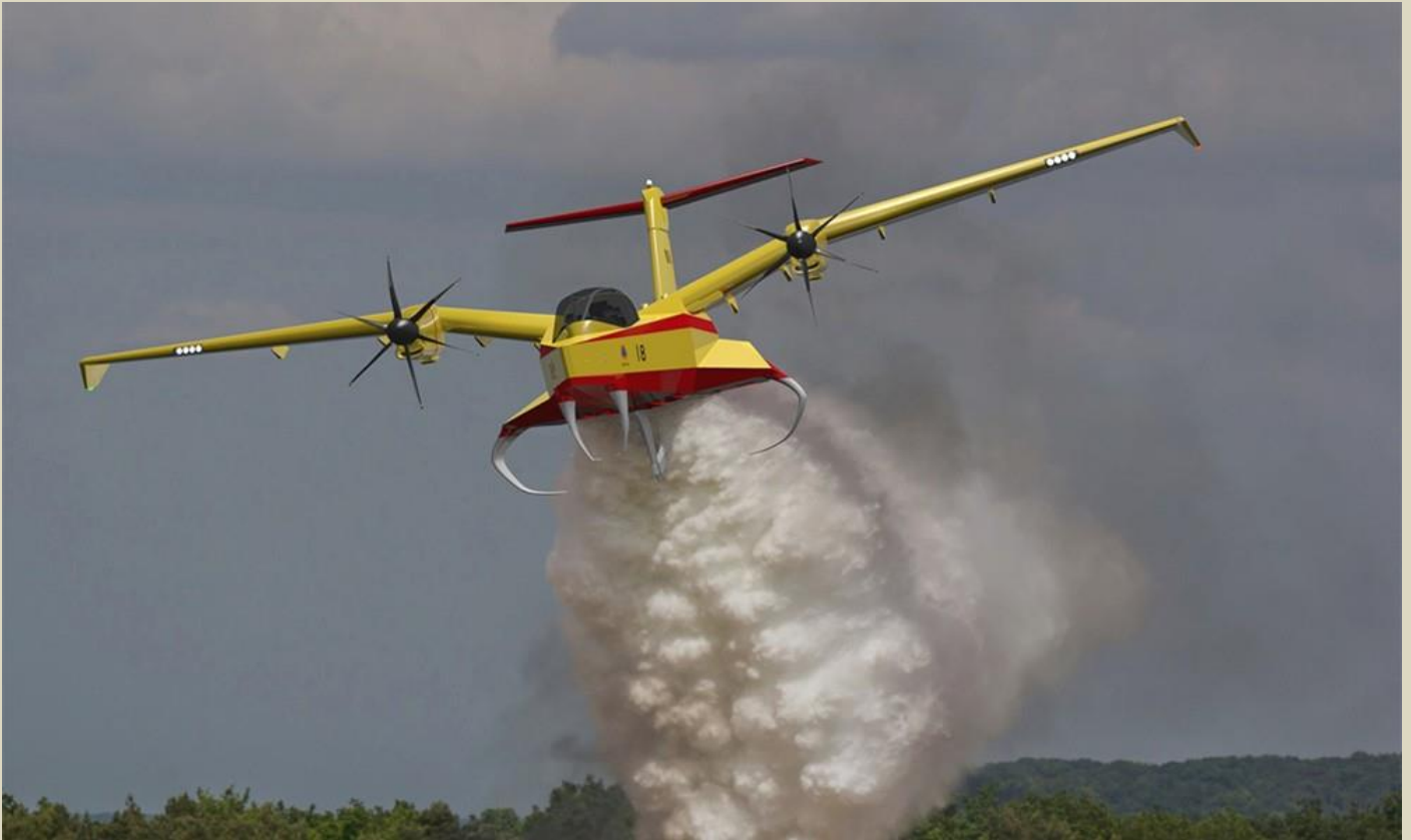
Seagle – hydrofoils; two tanks; anti-corrosion materials; 360° cockpit
