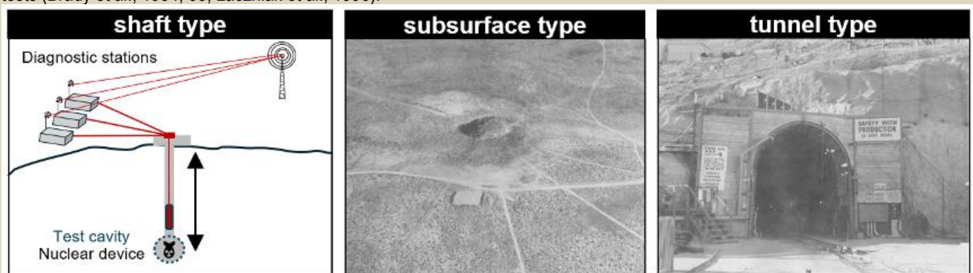
Figure 1. The three main emplacement types of underground nuclear tests. (Source: Shaft type illustrated by S. Park; subsurface and tunnel type pictures from Schoengold and Stinson 1997.)
